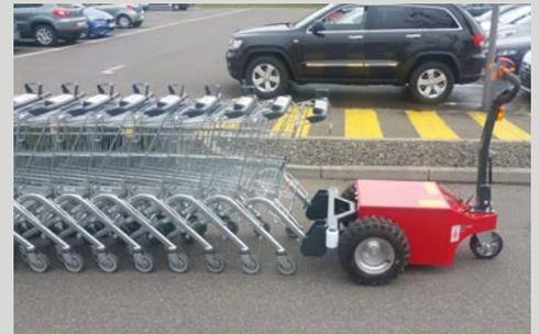
Shopping cart pusher model has maintenance-free AC motor, cart attachment and wireless remote
